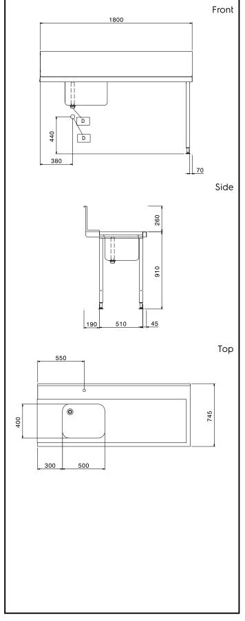
Handling System for Hood type Pre-wash Table with Bowl Right to Left, 1800mm
